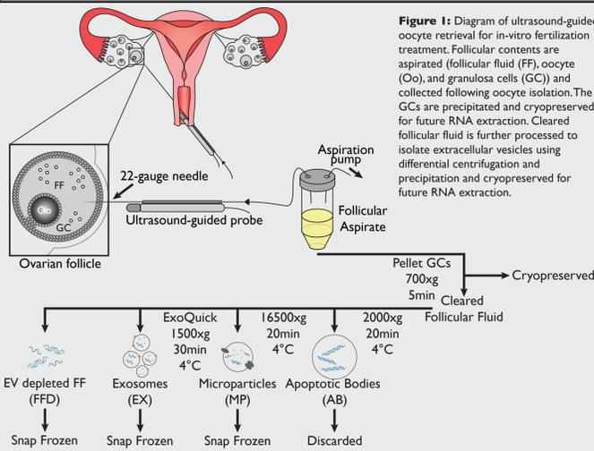
**Figure 1:** Diagram of ultrasound-guided oocyte retrieval for in-vitro fertilization treatment. Follicular contents are aspirated (follicular fluid (FF), oocyte (Oo), and granulosa cells (GC)) and collected following oocyte isolation. The GCs are precipitated and cryopreserved for future RNA extraction. Cleared follicular fluid is further processed to isolate extracellular vesicles using differential centrifugation and precipitation and cryopreserved for future RNA extraction.
